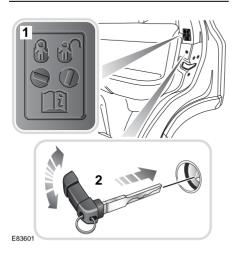
Child safety locks are fitted to the rear doors to allow you to prevent accidental opening of the doors when the vehicle is in motion.
